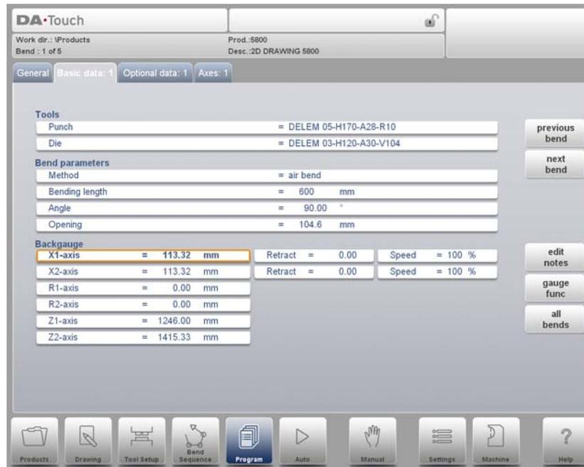
If Gauge Func is pressed, a window appears with several programmable parameters. These parameters serve to program the desired finger positions for a certain bend. The necessary axis positions that are necessary for this bend are calculated from the programmed finger positions
