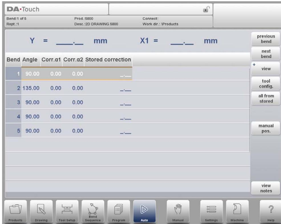
In this window the corrections of all bends are shown. You can browse through all corrections and change them as you see fit. If a correction for  $\alpha_1$  is entered then this value is copied to the correction for  $\alpha_2$ . Different corrections for  $\alpha_2$  can be entered in the field itself. The columns 'measured  $\alpha_1/\alpha_2$ ' are present if they are enabled through the parameter 'angle correction computation' in the Settings mode.
