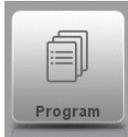
To create a new CNC-program or edit an existing CNC- program numerically.
