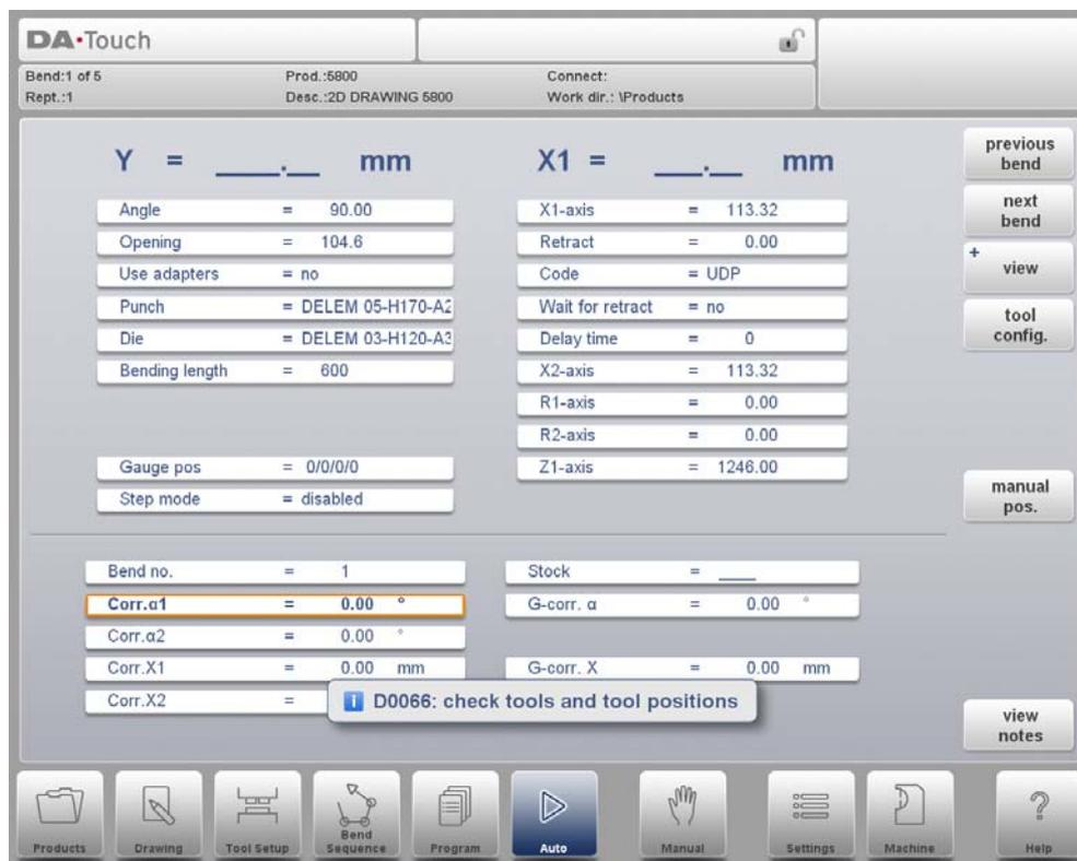
The automatic mode executes the program automatically bend by bend after pushing the Start button. When selecting a different product in Products mode, which is in the library and has already been used for production, one can immediately switch to Auto and start production. Every time after a different bending program is selected you must check your tools and tool positions in your machine. This is also indicated with a 'check tools' warning message when you enter the automatic mode.
